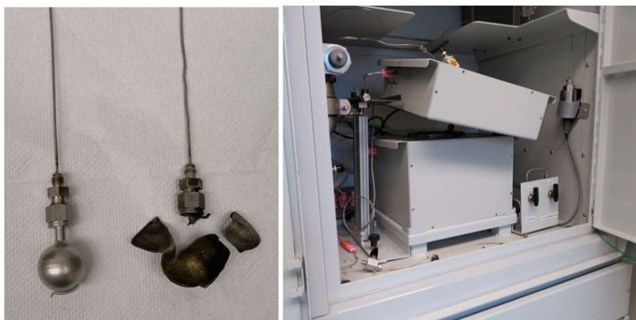
Figure 6. Pictures of (left) a ruptured Hastelloy C ARC cell and (right) the displaced ARC reactor housing resulting from the cell explosion.
