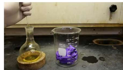
Fuming HNO 3 to nitrile gloves
